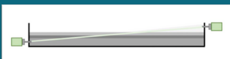
Figure 1 - Schematic of an optical phantom (grey) in a petri dish containing a hollow channel (green) with needles at the outer ends.
